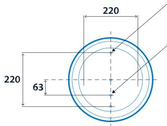
Recommended fixings - 4 x spot faces, drill as required
